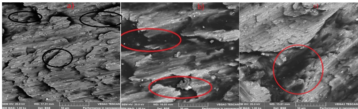
a. Wear fracture surface of the Epoxy matrix on a) Load of 10N b) Load 20N c) 30N
