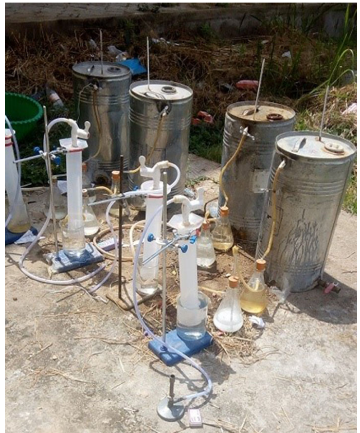
Figure 1. Fabricated digesters and experimental set-up.
